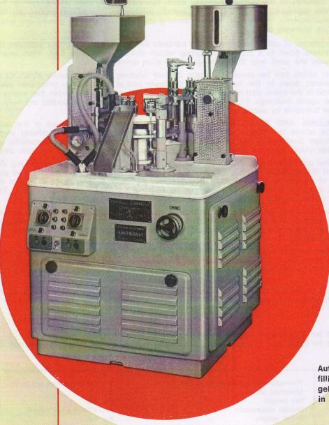
**Automatic machine for** filling and closing hard gelatine capsules in two-pieces
